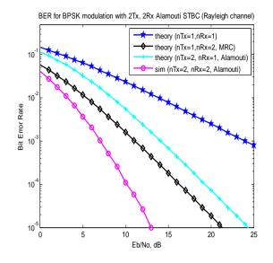
In this graph the value SNR of 11 y=y=4.9000e-05 but when we use transmit beamforming technique y=5.8000e-05 and also the value SNR of 15 then y=1.0000e-06 but by using beamforming y=4.0000e-06 and also the value SNR of 16 y=0 whereas by using beamforming y=1.0000e-06 and also the value SNR of 15 then y=1.0000e-06 but by using beamforming y=2.0000e-06 respectively.
