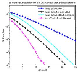
This graph shows the bit error rate for BPSK modulation with 2 Tx and 2 Rx antenna.
